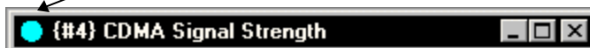
Figure 61 Title Bar Right-click on the symbol to open the Properties dialog box.
